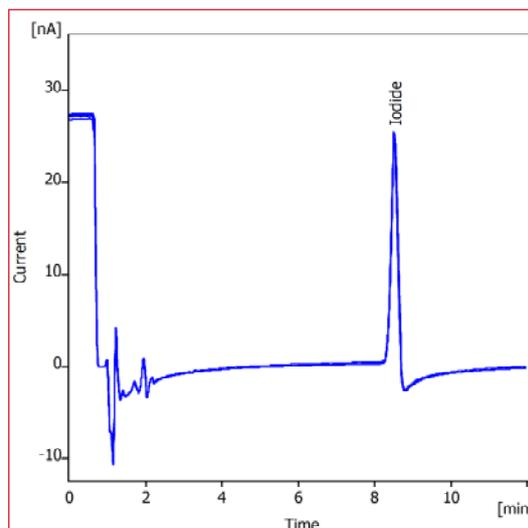
**Figure 5.** Overlay of 6 chromatograms of 5 μM (0.63 mg/L) potassium iodide in water, recorded with conditions given in Table 1.
