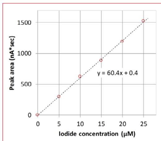
**Figure 6:** Reponse plot for iodide in water. Data based on analyses with conditions as given in Table 1.
