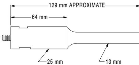
1/2" (13 mm) probe with replaceable tip\*
