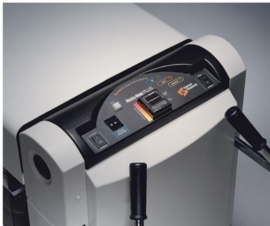
The easy-to-use controls on the Media-Mate panel allow one push to initiate a complete media measurement, deaeration, and dispense cycle, filling all 6 or 7 dissolution vessels in less than 5 minutes.
