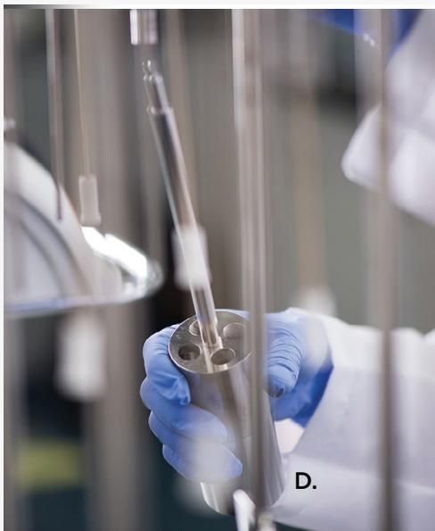
The Rotating Cylinder complies with USP <724> and holds patches up to 5 x 14 cm in size (f.). For larger patches up to 10 x 14 cm in size, a Rotating Cylinder with Extension (d.) is available (both pieces are matched and must be purchased together). The Rotating Cylinder and Extension are serialized and come with a Certificate of Conformance.
