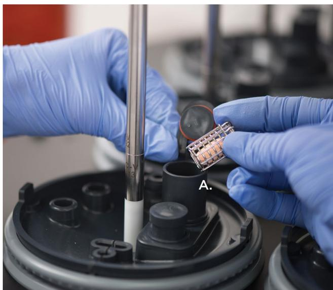
Sinker loaded into an Easi-Lock ADD cover for automatic dosage delivery.
