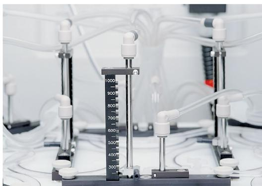
Volume change adjustment provides quick and easy settings from 250 mL to 1,000 mL in 50 mL increments. Rapidly fill 6 or 7 vessels in Hanson, Agilent, VanKel, Distek, Erweka, and other brands of dissolution testers.
