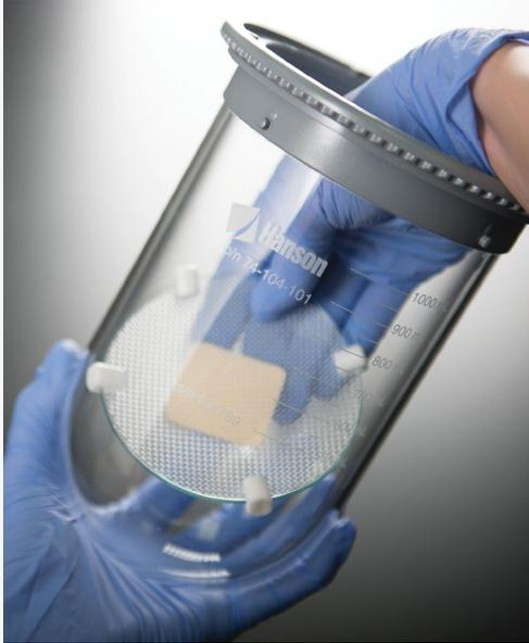
The Hanson Transdermal Sandwich (USP App. 5) is a convenient disk assembly recommended by the US FDA for testing patch dosage forms in a standard dissolution test station. It consists of a glass watchglass (on which the patch is placed, delivery side up), a 17 mesh PVDF screen to hold the patch, and PVDF clips to hold the disk assembly together.
