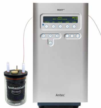
Figure 8: SynthesisCell (80 mL reaction vessel) with ROXY Potentiostat
