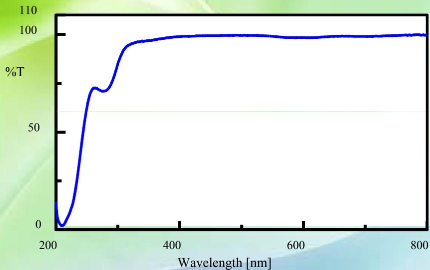
**Fig 5. Spectrum of hard contact lens sample**
