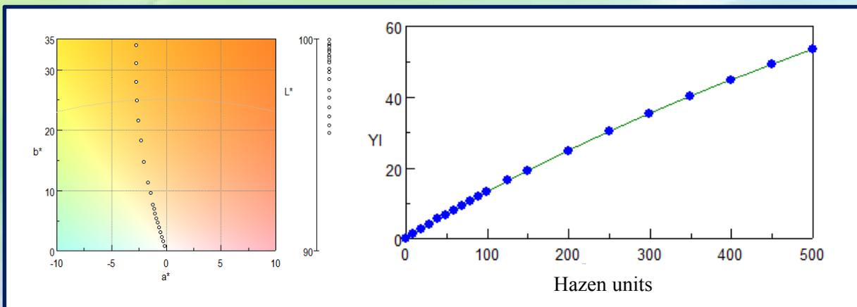
**$L^*a^*b^*$  color system with standard solution coordinates plotted**
