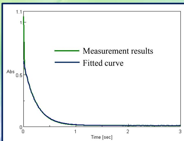
**Figure 3 Time-course measurement results and fitted curve for sample absorbance at 604 nm**
