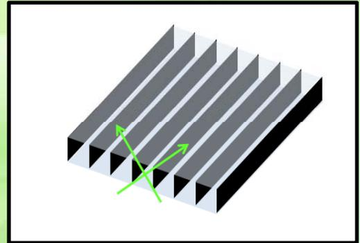
Fig. 1 Structure of louver layer
