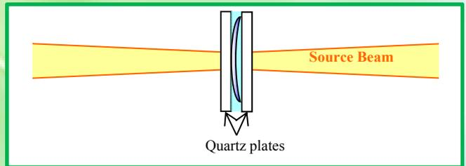
**Fig2. Contact lens between quartz plates**
