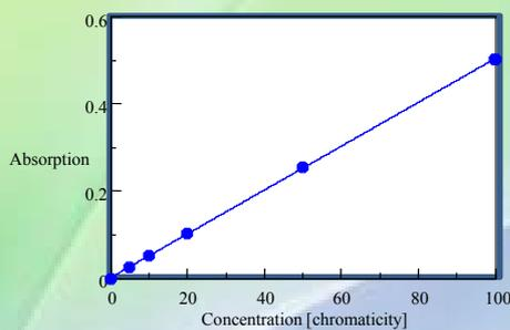
**Figure 2. Turbidity calibration curve (Transmission measurement method)**
