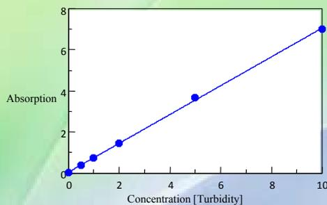
Figure 4. Turbidity calibration curve (integrating sphere photoelectric spectroscopy)
