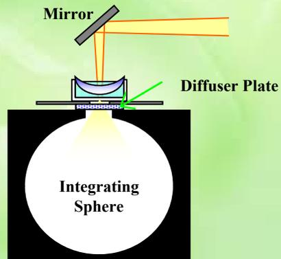
**Fig4. Sample placed on the horizontal integrating sphere**
