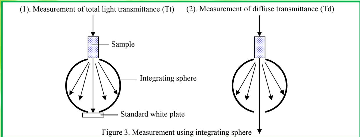
Figure 3. Measurement using integrating sphere
