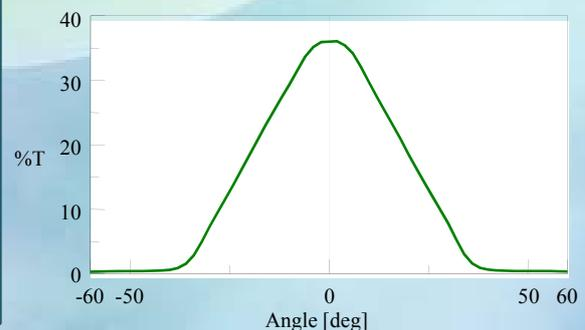
**Fig. 7 Angle dependence of transmittance spectra at 550 nm**
