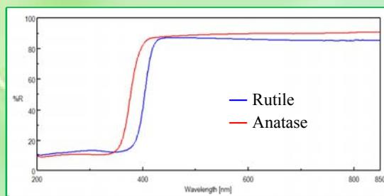
Diffuse transmittance spectrum for TiO2
