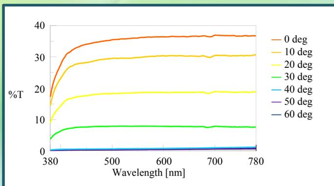
**Fig. 6 Transmittance spectrum at every 10° from 0° to 60°**
