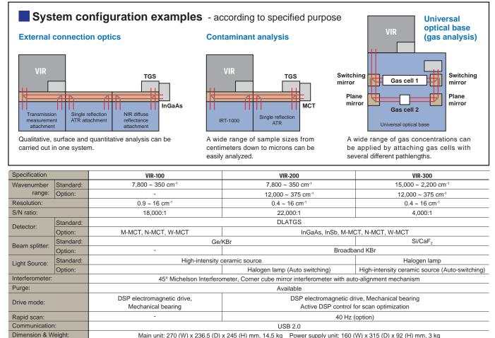
Main unit: 270 (W) x 236.5 (D) x 245 (H) mm, 14.5 kg Power supply unit: 160 (W) x 315 (D) x 92 (H) mm, 3 kg
