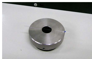
Photo 3. Holder for reflection measurement
