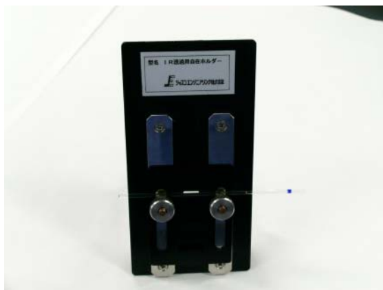
Photo 2. Holder for transmission measurement
