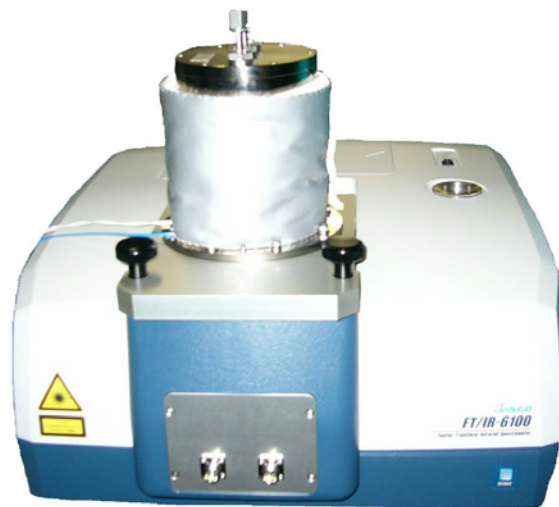
Fig. 1 Full vacuum type FT-IR gas analysis system (10 meter cell)
