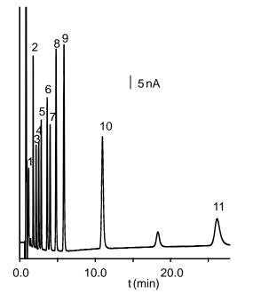
Fig. 2. Analysis of a standard mixture of phenol.
