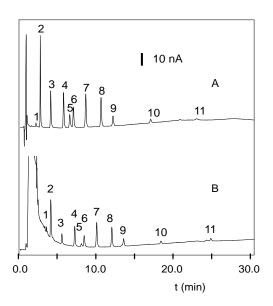
Fig. 3. Improvement in determination limit by large volume sample injection. Injection volume and concentrations for each phenol are A: 20  $\mu$ l (200 ppb) and B: 2 ml (2 ppb).
