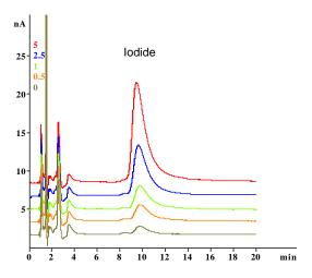
Fig. 2. Standard addition analysis of iodide in diluted (factor 10) and filtrated urine using ECD with a silver working electrode (20  $\mu$ L). From top to bottom: urine with addition of 5, 2.5, 1, 0.5 and 0  $\mu$ mol/L potassium iodide. Peak height of iodide (at t=10 min) corresponds to a concentration of 4  $\mu$ mol/l in urine.
