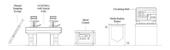
Figure 5. Manual diffusion cell system.
