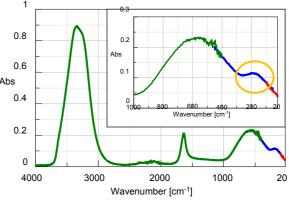
Figure 2: ATR spectra of pure water (Upper right: Enlargement below 1000 cm<sup>-1</sup>)
