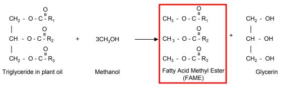
Fig. 1: Reaction pathway from vegetable oil to FAME
