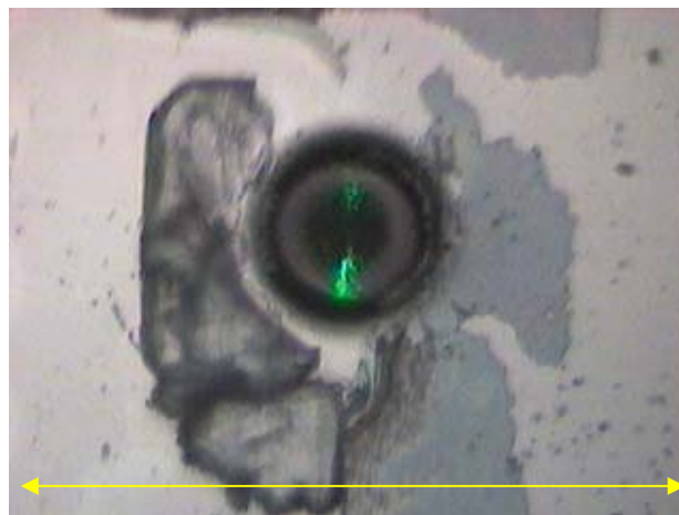
Figure 1. Microscope view of the inkjet hole using a 20X lens. Scale (yellow) is 250 \mu\text{m} . The green spot is the laser focus.
