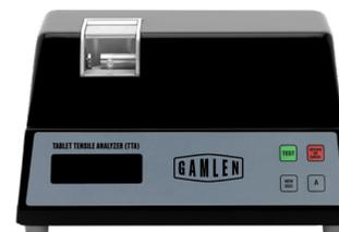
The Gamlen TTA (Tablet Tensile Analyser) measures tablet diameter and breaks the tablets to measure tablet tensile fracture stress. Values are automatically captured by the software.
