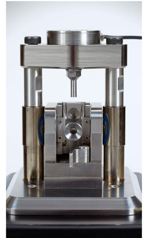
The patented integrated detachment mechanism consists of a rotating die and simple lever. This allows compaction, detachment and ejection operations to be carried out with no need for awkward re-configuration.
